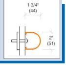
Retainer: Continuous Aluminum Dimensions: 1-3/4"D x 2"H
