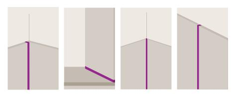
Corners can also be produced using neutrally crosslinking silicone.
