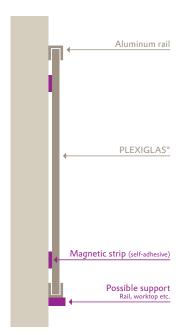
Principle: self-adhesive magnetic strip (types A and B).
