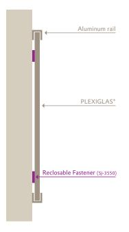
Principle: self-adhesive, flexible press-on fastener system.
