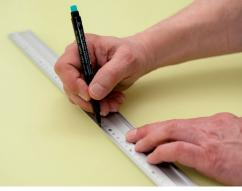
Always mark recesses and apertures on the masking film and predrill holes in the corners of cut edges.
