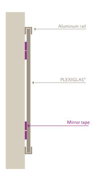
Principle: Key and lock insertion. Lock is fastened to wall by bonding or with screws
