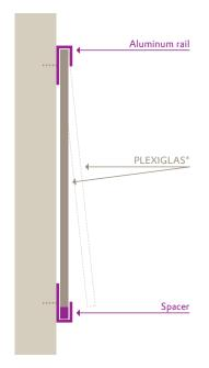
Principle: Aluminum U-rail with long leg Fasten rails by bonding or with screws. Place the spacer in the lower profile.
