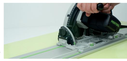
A guide rail or parallel stop is used to safely guide the circular handsaw.
