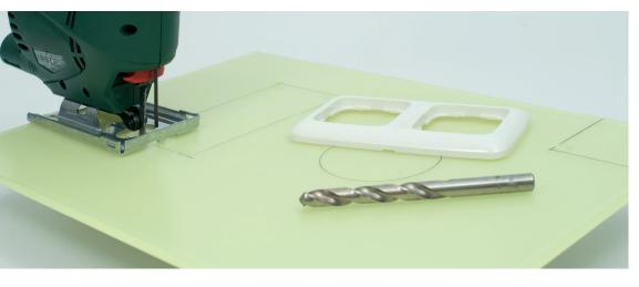
Always predrill recesses and apertures in the corners of cut edges and cut them out with a jigsaw or overhead template router.
