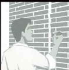
Texture the Mastic with slight touches, **not brush-strokes**. Use a brush "paletina" or a No.01 paintbrush that must be cleaned to remove the excess of Mastic.
