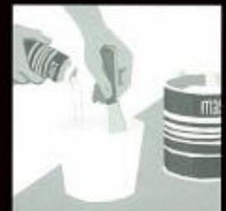
Prepare the Mastic adding 1-2% of the weight in Accelerator. Mix the ingredients.
