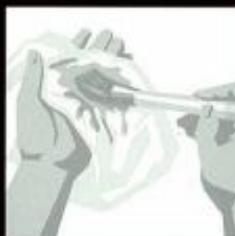
Once the Mastic is dried, paint with the Mastic colour, draining the brush in a rag to avoid dripping.
