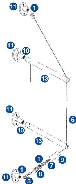
**#1806** - Designed for shelving, panels etc. Rod extends 260mm from wall. Minimum shelf width 215mm (when used horizontally)
