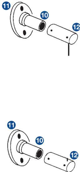
**#1802** - Designed to display vertical panels 45mm from wall (mount wall fittings pull cable through bottom wall spacer and tension with pliers, then tighten up with grub screws).
