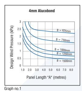
Graphs no.1 and no.2 indicating maximum permissible panel lengths are based on the applicable design wind load (kPa) and required panel width (B). Maximum permissible bending stress = 55 MPa.
