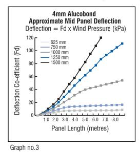
Graphs no.3 and no.4 indicating the approximate mid-panel deflection for different panel lengths and widths and are based on the results of extensive testing and research.
