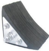
Laminated recycled tire rubber pads assembled on 3/4" (19.1mm) bolts and compressed between 1/4" (6.35mm) steel plates. Positive grip - contoured to fit curvature of tire. Ideal for heavy utility trucks and equipment, large cable rolls and buses.
