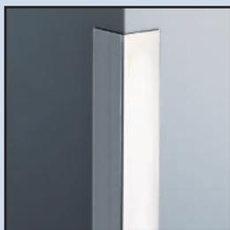
Our mill finish aluminum corner guards are easy to install and come in wing sizes from 1" to 3". They come standard with adhesive, or can be pre-drilled for mounting with mechanical fasteners. Customize the look you need with lengths up to 10'. Also available in custom angles and wing sizes.
