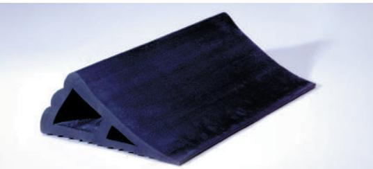
Heavyweight design used to contain metal pipes, rolls, cable, and light trailers. Smooth surface prevents damage to outside layers of paper rolls. EPDM rubber compound provides outstanding durability and weather resistance. Available in any length up to 12'0".
