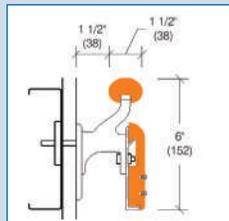
Foundation Series handrail offers versatility and flexibility by "building" the look you desire. Combine a round vinyl handgrip with a 4" vinyl bumper. Features: ADA Compliant, Class A fire rating, Molded returns - with hardware, Molded outside corners - with hardware.
