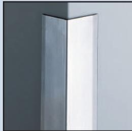
Our stainless steel corner guards come in type 304, 316 or 430 Stainless Steel with #4 Satin finish and a variety of radii and corner angles with custom angles and wing sizes also available. Combine with our CRS-100 for a coordinated stainless steel design that provides heavy duty impact protection. Installation is easy with our standard adhesive or optional pre-drilled holes for fasteners.
