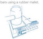
It is recommended that the top glazing bar is secured to the rafter with screws (gauge not exceeding 12g) at no greater than 1200mm apart. Once the next sheet is installed the second and subsequent top glazing bars can be fitted.
