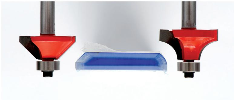
Routers with ball bearing bits require no other guides and can be used both for straight and curved edges.
