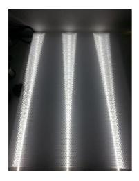
Abstand LED zu LED 200 mm Abstand LED zu AIR-board 25 mm distance LED to LED 200 mm, dist. LED to AIR-board 25 mm
