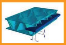
Tongue & groove connection for panel joints without profiles; specially designed for standard aluminium booth construction profiles.
