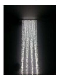
Abstand LED zu LED 50 mm Abstand LED zu AIR-board 25 mm distance LED to LED 50 mm, dist. LED to AIR-board 25 mm
