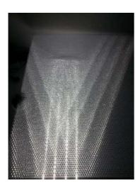
Abstand LED zu LED 50 mm Abstand LED zu AIR-board 200 mm distance LED to LED 50 mm, dist. LED to AIR-board 200 mm
