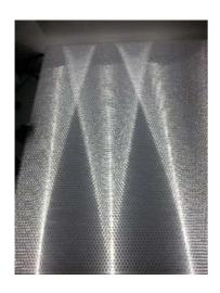
Abstand LED zu LED 200 mm Abstand LED zu AIR-board 100 mm distance LED to LED 200 mm, dist. LED to AIR-board 100  $\,$
