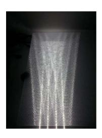
Abstand LED zu LED 50 mm Abstand LED zu AIR-board 100 mm distance LED to LED 50 mm, dist. LED to AIR-board 100 mm
