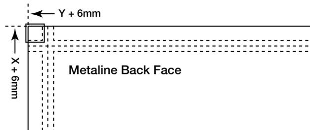
1. Router the back of the sheet as per previous detail for rolled edges allowing the two passes to criss-cross over the corner edge.
