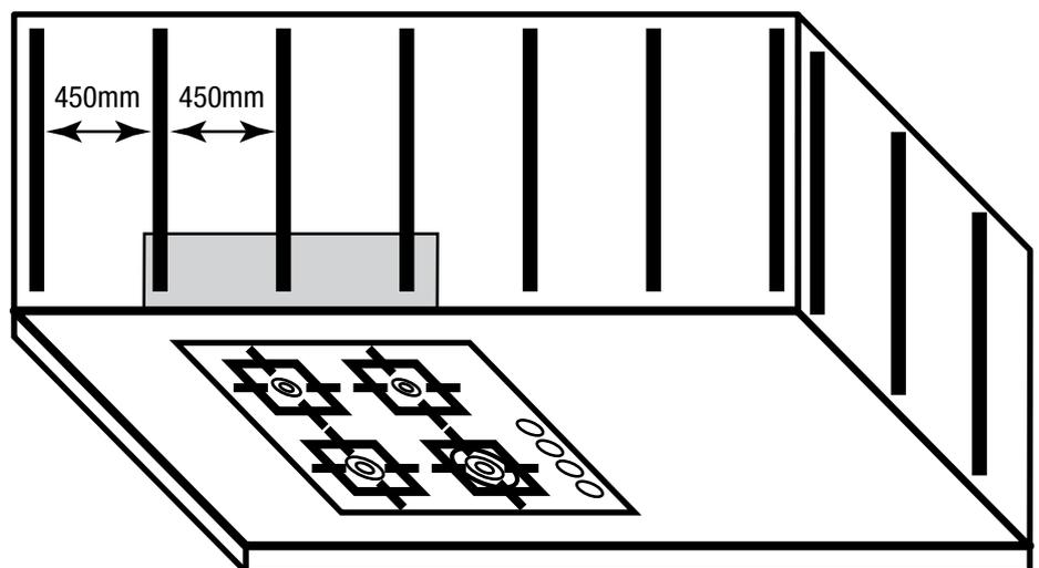
Figure 9: Application of double-sided tape to the wall
