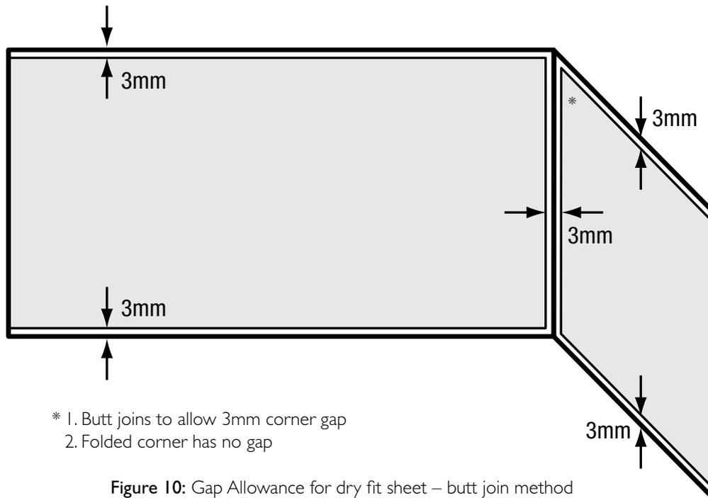
Figure 10: Gap Allowance for dry fit sheet – butt join method
