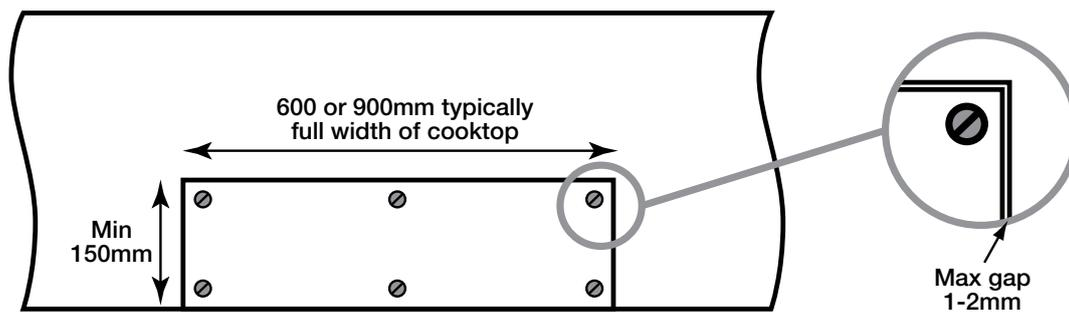
Figure 7: Detailed installation of mineral board with self-tapping screws showing allowable gaps
