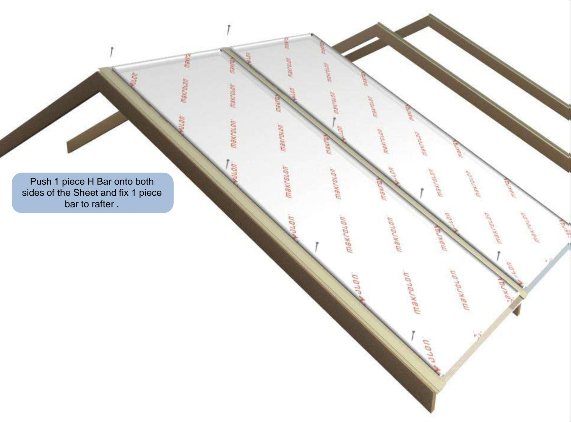
A 3D perspective diagram showing a white sheet of material with a repeating red 'MAKROLON' logo being installed on a wooden rafter. A brown H-bar is being pushed onto the edge of the sheet. The sheet is held in place by several screws. The rafter is supported by a wooden beam. The diagram illustrates the step of securing the sheet to the rafter with an H-bar.
