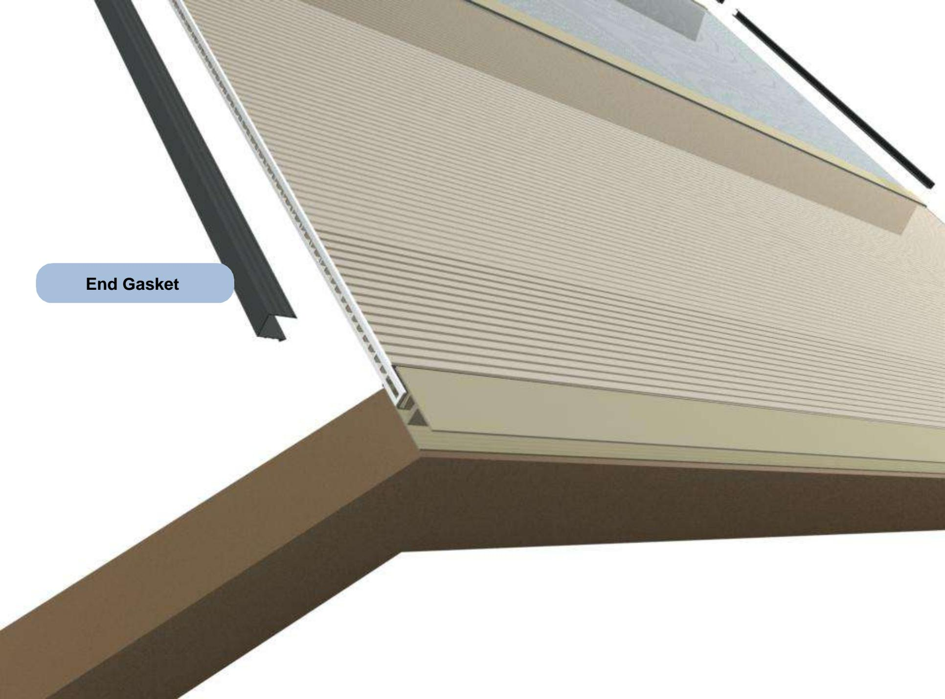
The diagram illustrates a cross-section of a roof assembly. At the top, a dark grey metal roof panel is shown. Below it is a layer of insulation with a blue textured surface. A white metal batten is positioned horizontally across the insulation. A black metal end gasket is being shown being inserted into a groove in the white batten. The roof assembly is supported by a brown structural member. The label 'End Gasket' is placed in a blue rounded rectangle on the left side of the image.
