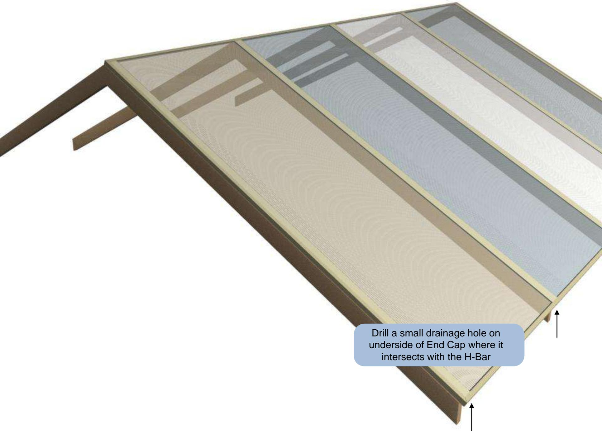
Drill a small drainage hole on underside of End Cap where it intersects with the H-Bar
